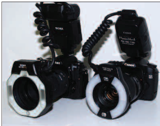
Figure 1. The Nikon D300 and Canon 40D digital SLR cameras (both shown with a macro lens and ring flash) can be used for more accurate doctor-technician communication.
